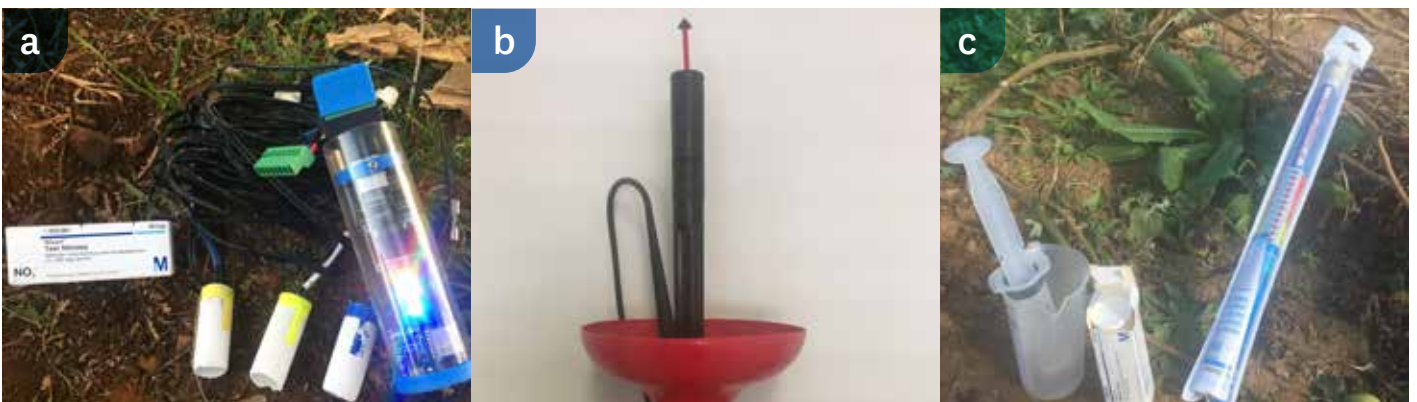
Figure 3. (a) Nitrate strips (left), Chameleon soil-water sensors (center), and sensor reader (right); (b) WFD to capture drainage water for monitoring of nitrate and EC; and (c) syringe (left), nitrate strips (center), and EC meter (right) for sampling the water collected in the WFD (photos: Manuel Magombeyi/IWMI).
