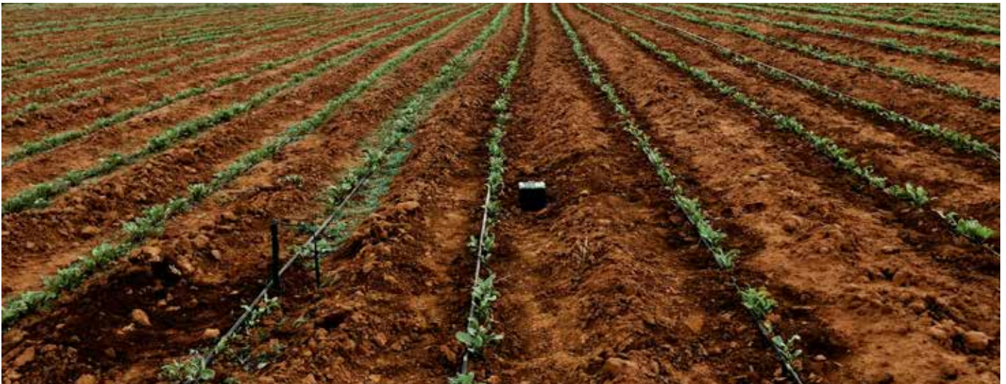
Figure 2. Wetting Front Detector and soil-moisture (Chameleon) sensor installed in a field with beetroot in Mogobane irrigation scheme, Botswana (photo: Manuel Magombeyi/IWMI).
