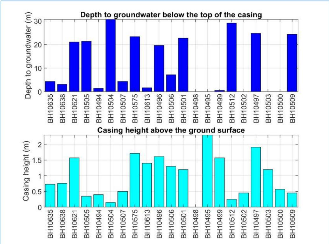
**Figure 23:** Depth to groundwater and casing height for the hydro-censuses observation boreholes. Boreholes with depth to groundwater close to zero are artesian wells.
