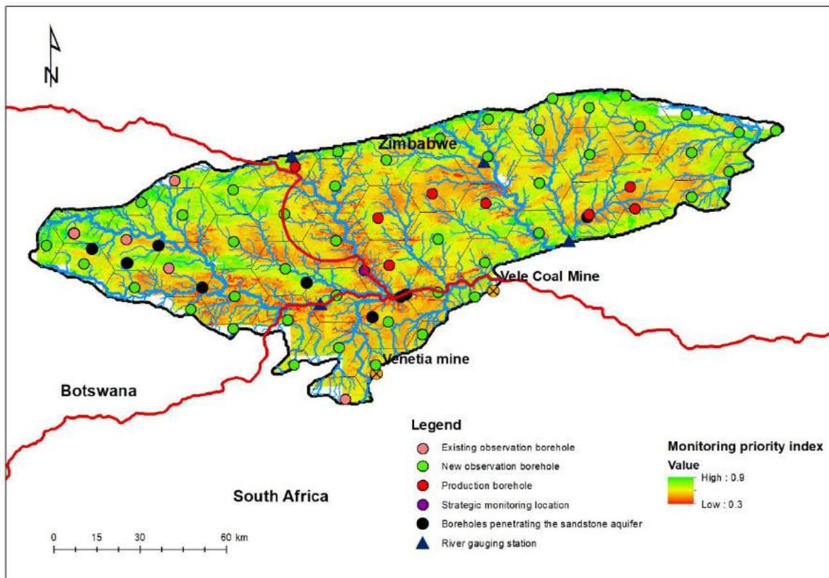
**Figure 27:** Optimal monitoring boreholes for the Tuli Karoo Aquifer overlaid with existing monitoring boreholes tapping the sandstone aquifer and monitoring priority index.
