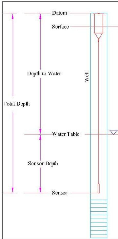
**Figure 22:** Typical data logger installation depths
