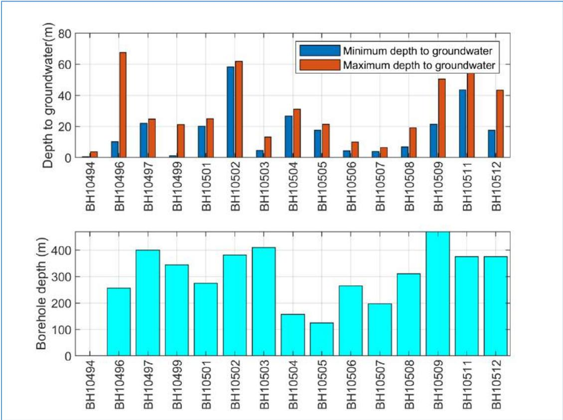
**Figure 9:** Borehole depth, minimum and maximum depth to groundwater in the Botswana portion of the Tuli Karoo Aquifer
