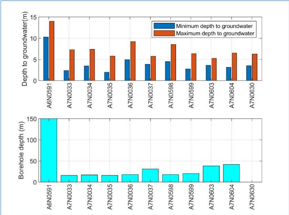
**Figure 10:** Borehole depth, minimum and maximum depth to groundwater in the South African portion of the Tuli Karoo Aquifer
