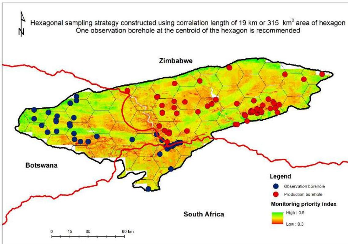
**Figure 26:** Hexagonal sampling grid over laid with monitoring priority index map and existing monitoring and production boreholes
