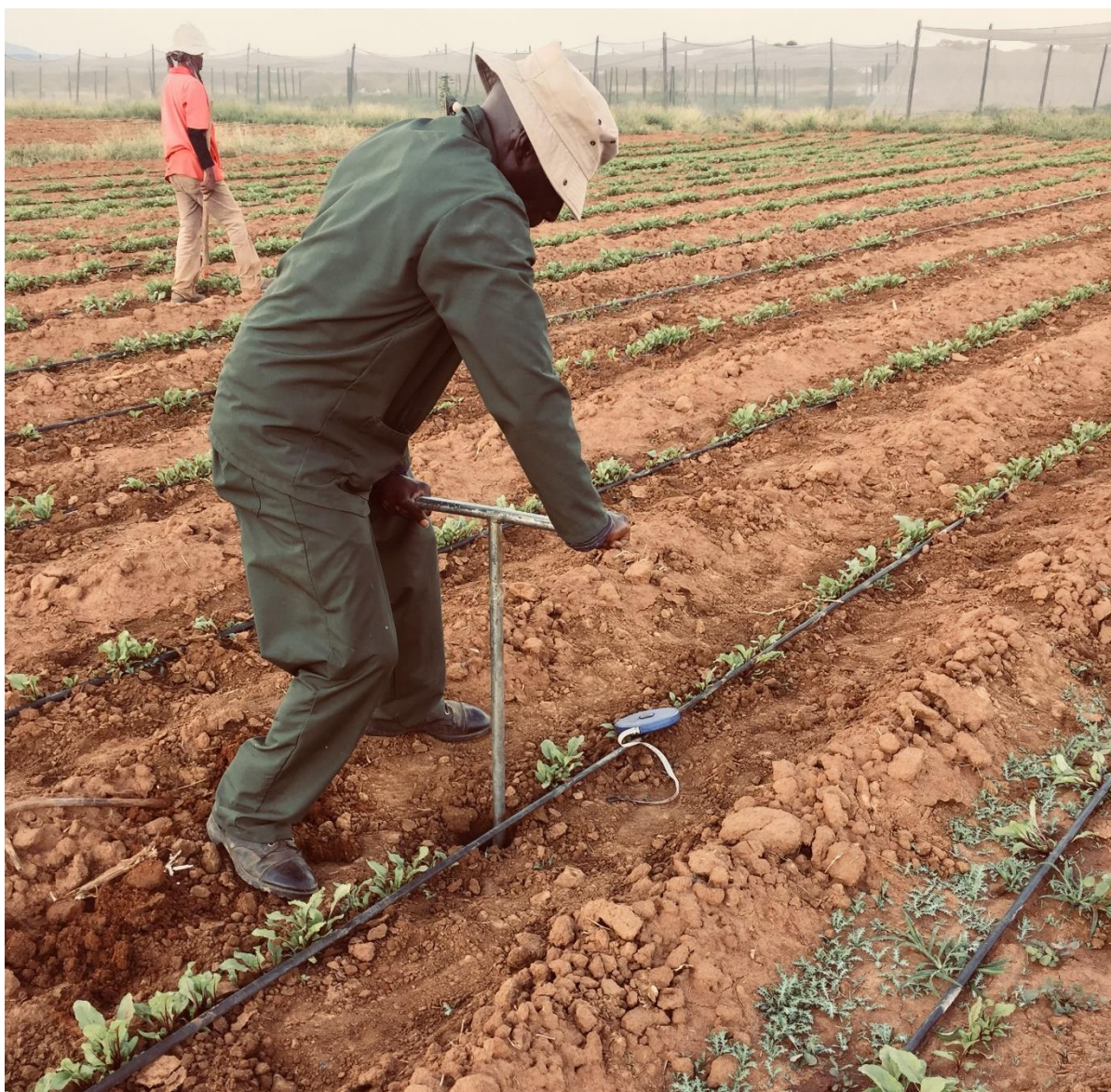
Photo. Chameleon sensor installation in beetroot crop at Mogobane Irrigation Scheme in Botswana
