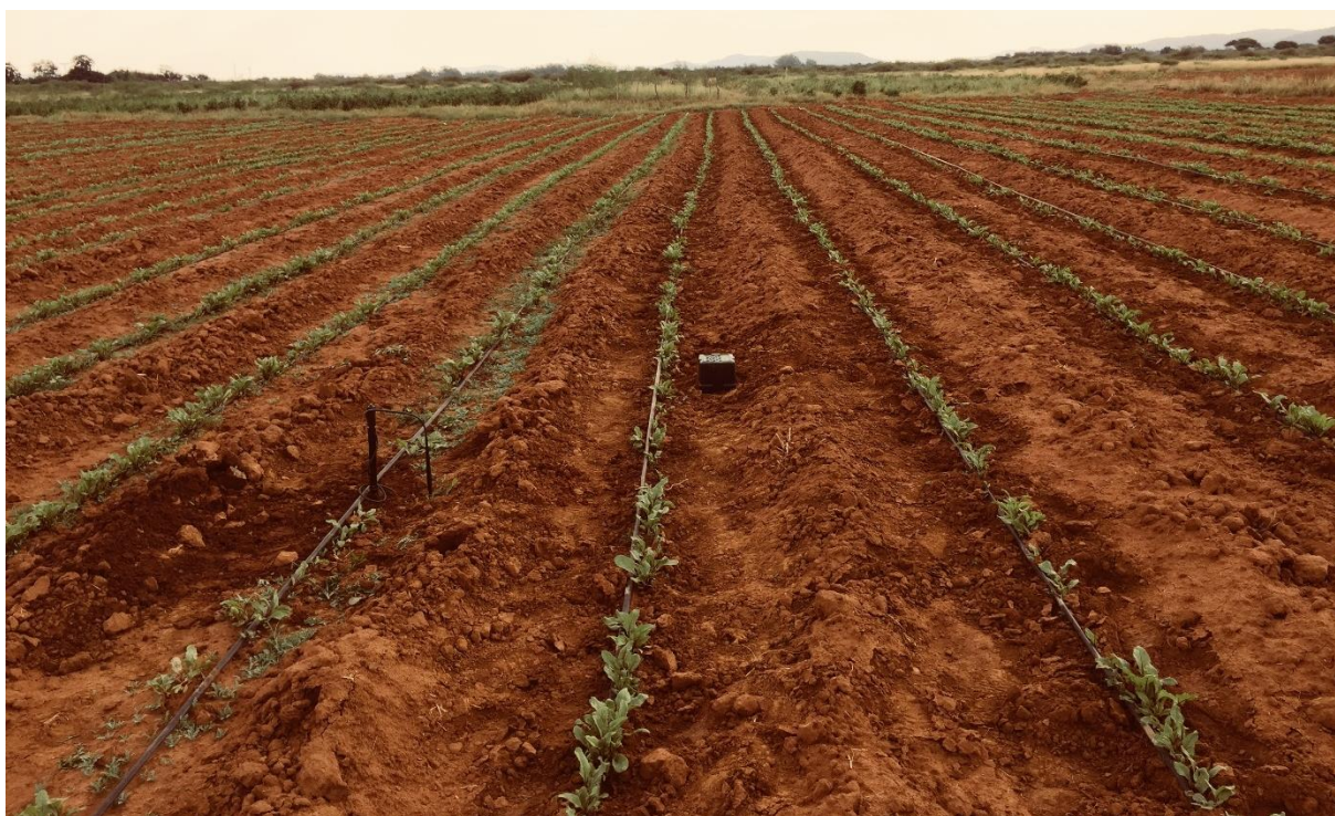
Photo. Chameleon sensor and wetting front detector installed in beetroot crop at Mogobane Irrigation Scheme in Botswana
