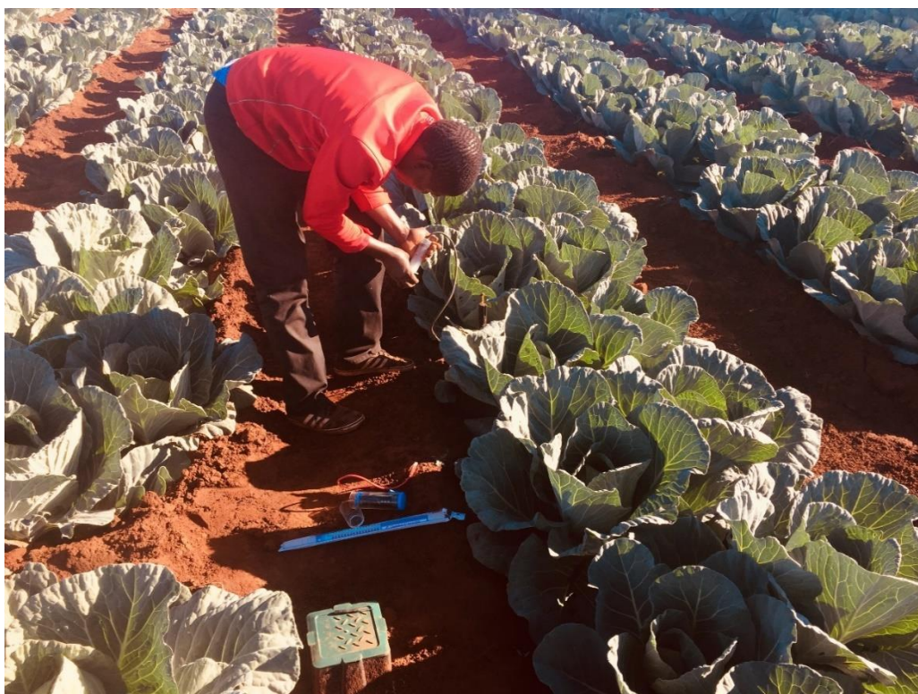
Photo. A youth farmer collecting drainage from a wetting front detector and taking readings from a chameleon sensor and electrical conductivity meter for cabbage crop at Motlhaka Irrigation Scheme in South Africa
