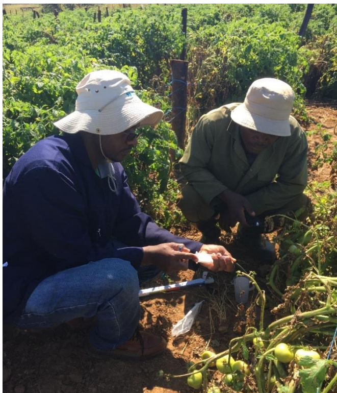
Photo. Farmer training on draining the wetting front detector and taking readings from a chameleon sensor
